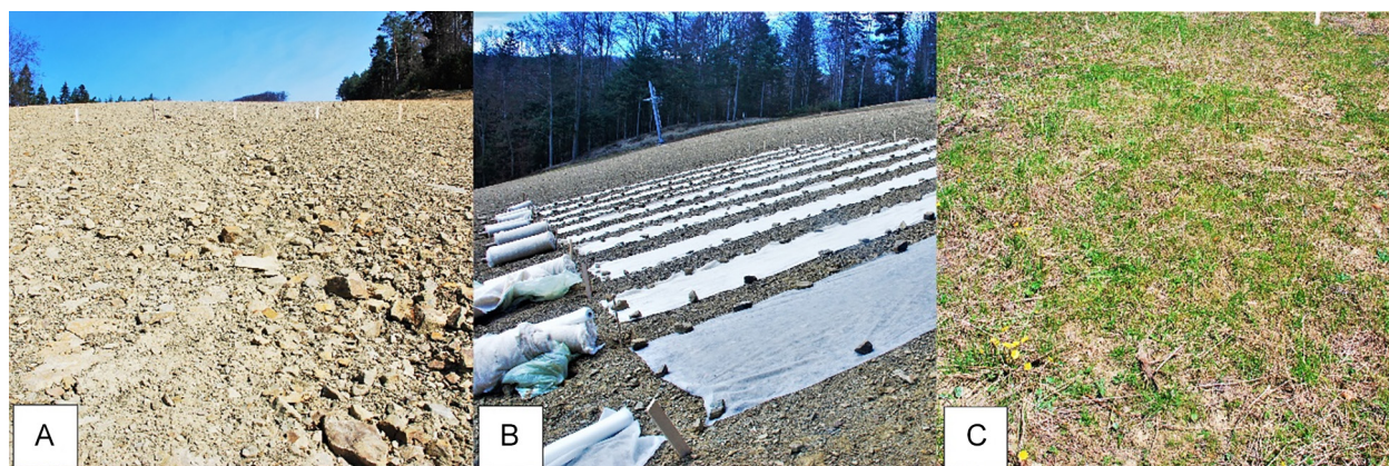
Fig. 1. Experimental design: A) the slope before the start of the field test; B) construction of the experimental plots; C) turf formation one year after the start of the experiment (photo by P. Kacorzyk)
